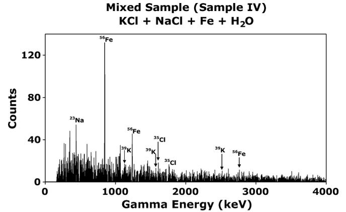
Fig. 5. Gamma energy spectrum from a mixed sample of 2.5 g KCl, 2.5 g NaCl and 5 g Fe in 40 g  $\text{H}_2\text{O}$ . Peaks are seen for each of the elements in the sample.
